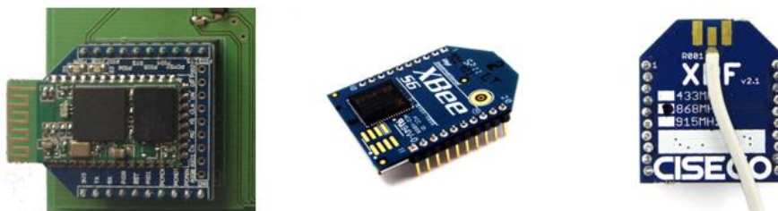
Figure 9 (from left to right): Bluetooth Bee module plugged in the ICSCorsair XBee slot, Wi-Fi XBee module, RF XBee module
