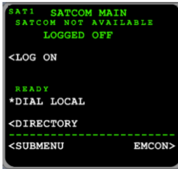
Figure 17: The SDU (Level D) Interacts with the MCDU (Level A Component Present in the Cockpit)
