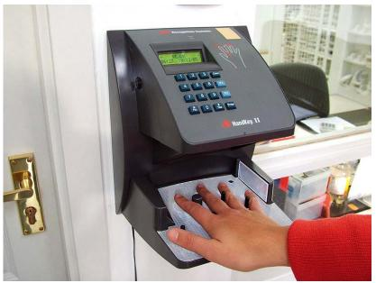
The addition of a 45 degree mirror allows them to add a check on the 3<sup>rd</sup> dimension.
