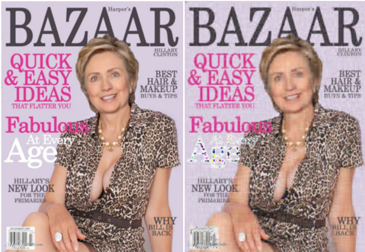
Figure 22. Photoshopped image with Hillary Clinton's head (left) and resolved using 5% of wavelets (right).
