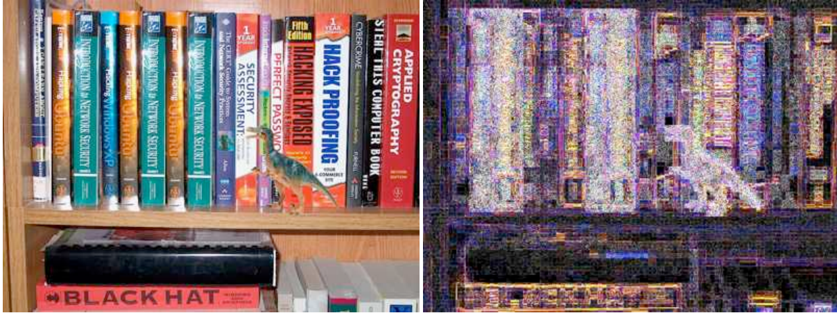
Figure 16. The first resaved image (75%) was modified. The 95% ELA identifies the modified areas: books were copied on the shelf and a dinosaur was added.
